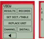
INSTALL FIRMWARE 1. CONNECT USB CABLE 2. CHOOSE UPGRADE IN PC 3. WAIT FOR OK TO APPEAR HERE
